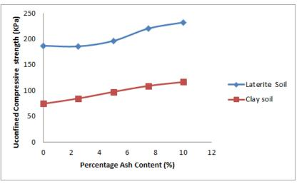
Fig-7: Unconfined compressive strength versus bagasse ash content
