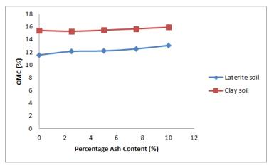
Fig-4: OMC versus bagasse ash content
