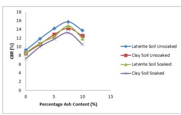
Fig-6: CBR versus bagasse ash content
