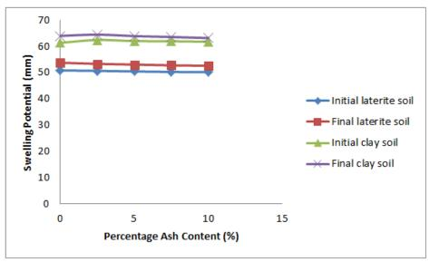
Fig-1: Swelling potential versus bagasse ash content
