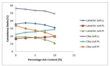
Fig-5: Consistency limits versus bagasse ash content
