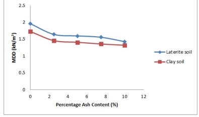
Fig-3: MDD versus bagasse ash content
