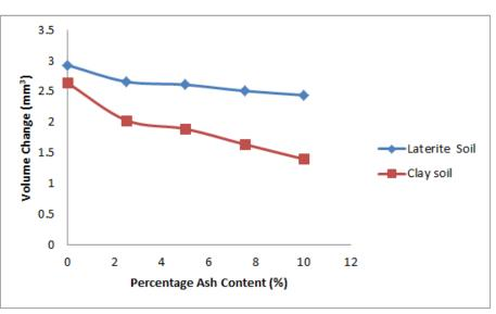
Fig-2: Volume change versus bagasse ash content
