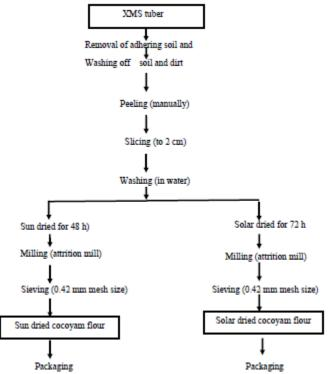
**Fig.1a:** Flow chart for the production of *Xanthosoma mafaffa* Schott (XMS) flour *Source:* Ukom and Okerue (2018)
