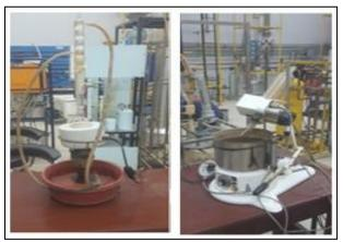
Fig.4: Soxhlet extractor and rotary evaporator
