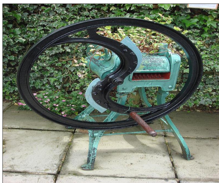
Figure 2: A hand powered chaff cutter (Source: Author, 2021)
