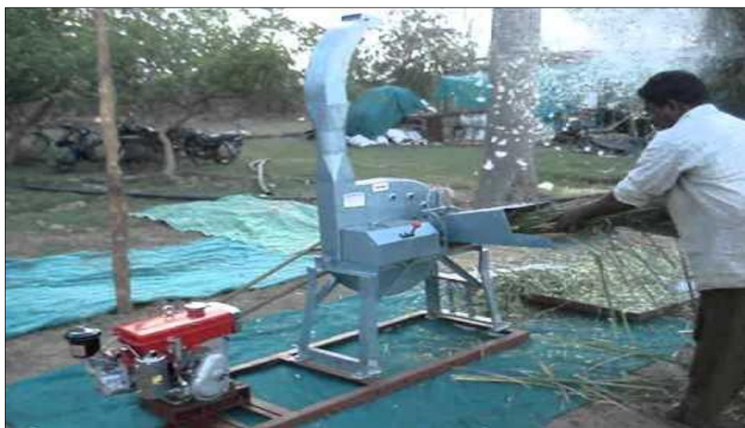
Figure 5: A fuel powered chaff cutter (Source: Author, 2021)
