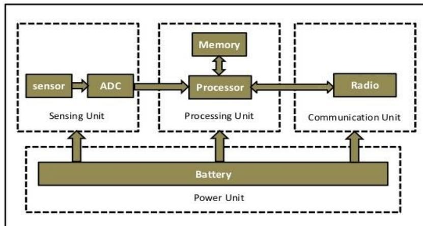
Fig 1.2: Components of sensor node
