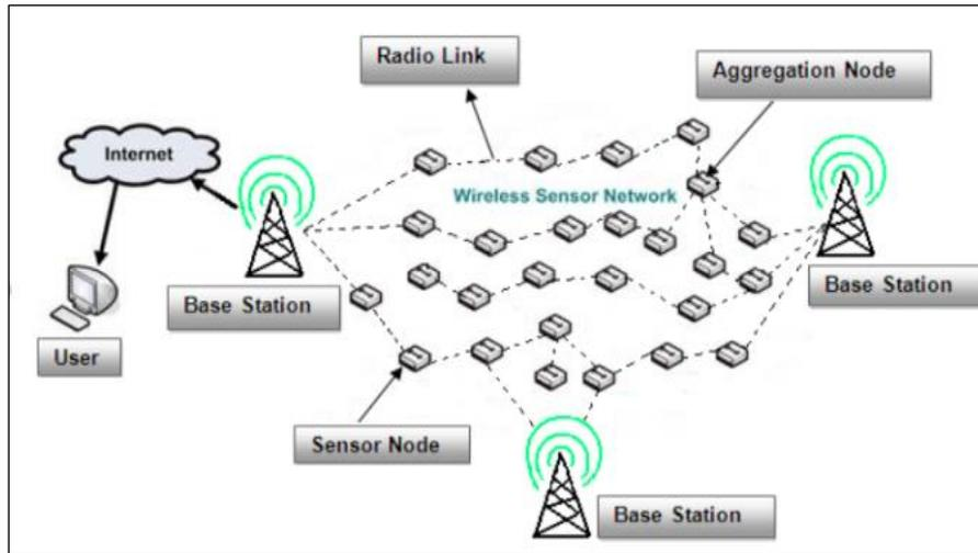
Fig 1.1: Basic Architecture of Wireless Sensor Network
