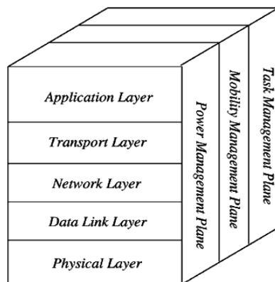
Fig 2.1: Wireless Sensor Network Protocol Stack
