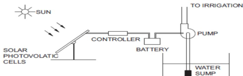
**Fig1: Experimental Set-up for Solar Water Pumping Based Drip Irrigation in Aerobic Rice**
