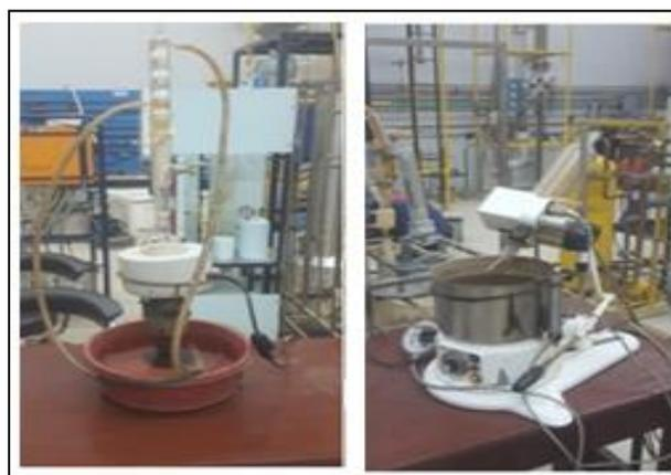
Fig.4: Soxhlet extractor and rotary evaporator
