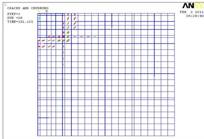
**Fig-11 Cracking in top surface near the column for slab SC1 by using ANSYS program**
