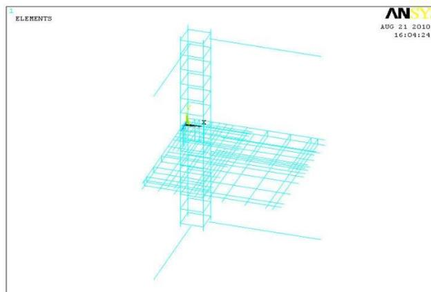
**Fig-4 Mesh of LINK8 elements for specimen**
