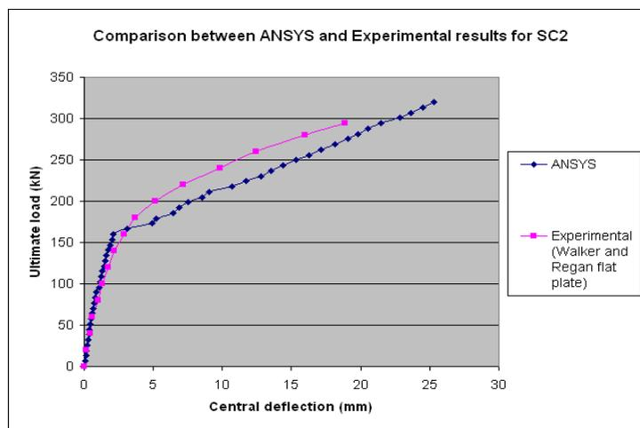
Fig-6 Load-Deflection response at mid-span of SC.2
