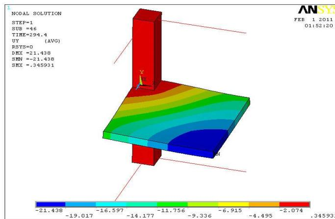
**Fig-9 Variation of UY (vertical displacement) along quarter of SC.2 at load equal to 98.5% of ultimate load**
