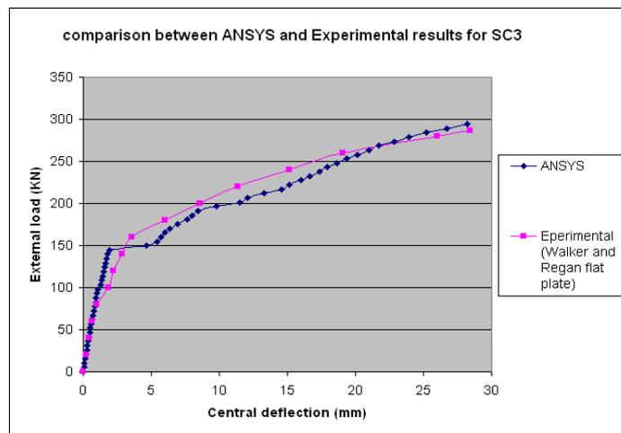
Fig-7 Load-Deflection response at mid-span of SC.3
