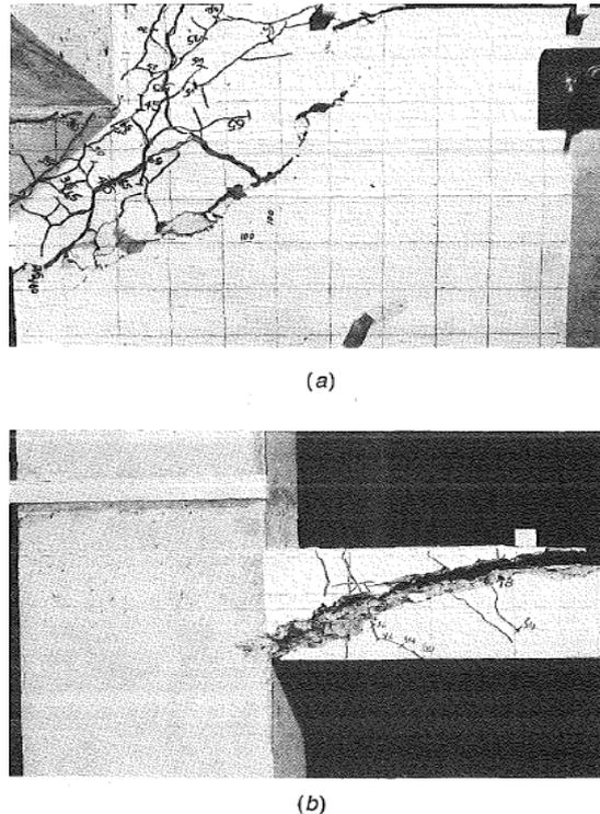
**Fig-16 Punching failure for slab SC1 (Walker, P. R., & Regan, P. E. 1987).**
