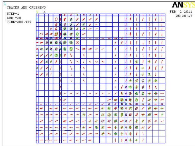
**Fig-13 Cracking in top surface for slab SC1 by using ANSYS program**
