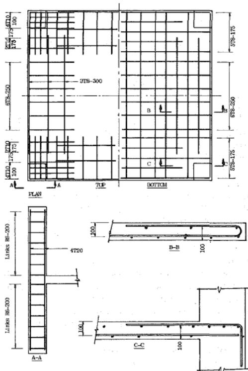
Fig-2 Reinforcement details for specimens (Walker, P. R., & Regan, P. E. 1987)
