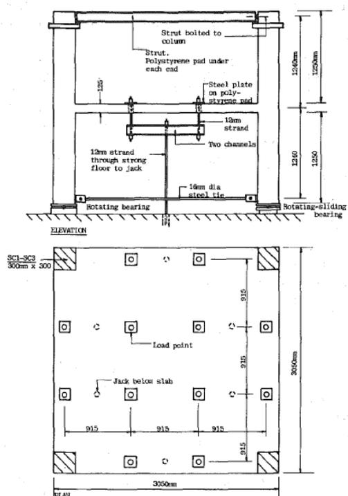
**Fig-1 Dimensions and load arrangement details for specimens (Walker, P. R., & Regan, P. E. 1987).**
