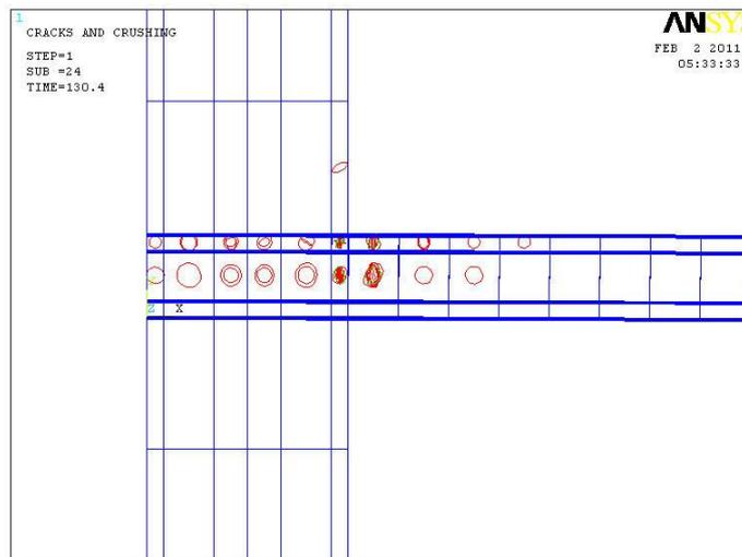
**Fig-12 Cracking in edges near the column for slab SC1 by using ANSYS program**
