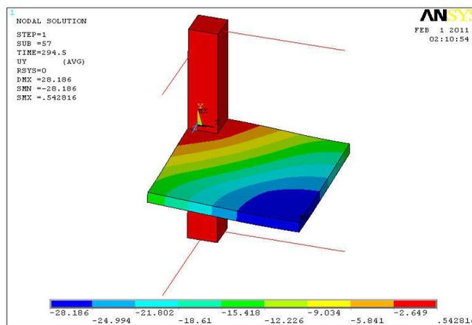
**Fig-10 Variation of UY (vertical displacement) along quarter of SC.3 at load equal to 99% of ultimate load**
