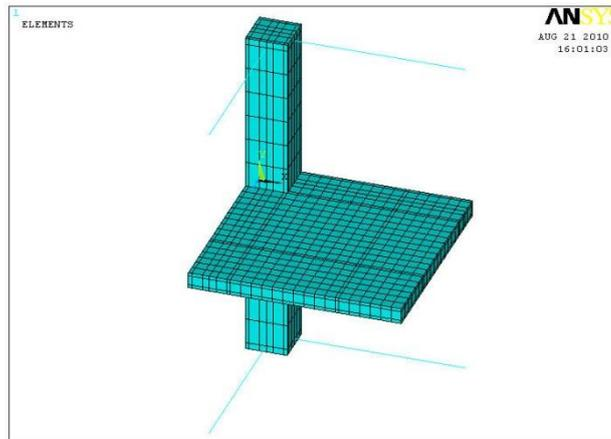
**Fig-3 Mesh of SOLID65 elements for SC.1, SC.2 and SC.3**
