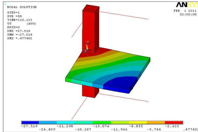
**Fig-8 Variation of UY (vertical displacement) along quarter of SC.1 at load equal to 96.6% of ultimate load**
