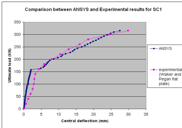
Fig-5 Load-Deflection response at mid-span of SC.
