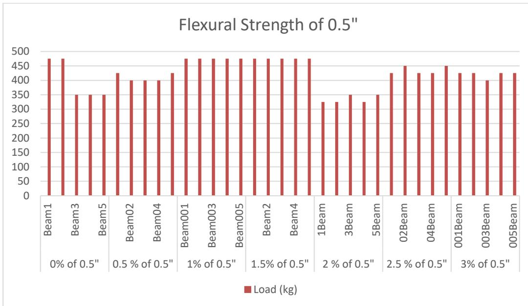
Figure 5: shows Flexural Strength of specimen at different loads with different percentage of waste tyre steel fibers of 0.5” size.
